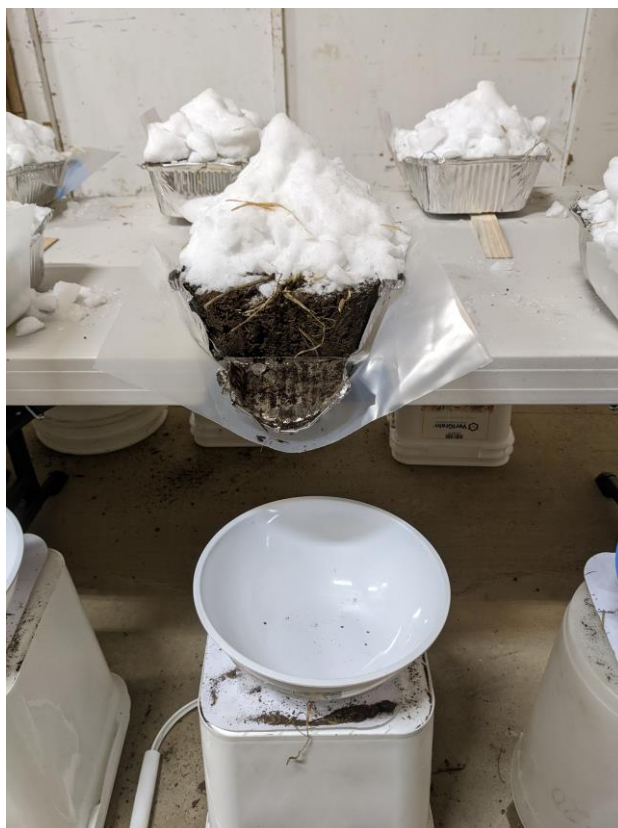
Figure 9. Snow addition to soil slab with container to catch run-off water (foreground) and wooden shim used to manipulate slope angle (background).
