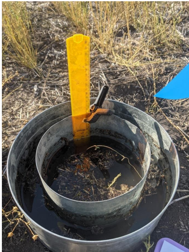
Figure 8. Double-ring infiltrometer used for water infiltration assessment.
